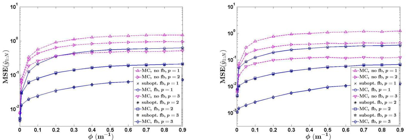
Fig. 4. Constant mean-signal scenario: Average MSEs of various estimators of  $\mathbf{y}_{1:N}$  as functions of  $\phi$ , for (a)  $K = 2$  and (b)  $K = 3$  quantization intervals and  $p \in \{1, 2, 3\}$  rounds.
