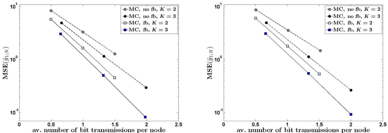
Fig. 10. Linear trend-surface scenario: Average MSEs of MC random-field estimators as functions of the average number of bit transmissions per node, for (a)  $\phi = 0.2 \text{ m}^{-1}$  and (b)  $\phi = 0.5 \text{ m}^{-1}$ .
