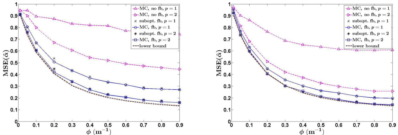
Fig. 3. Constant mean-signal scenario: Average MSEs of various estimators of  $\alpha$  as functions of  $\phi$ , for (a)  $K = 2$  and (b)  $K = 3$  quantization intervals and  $p \in \{1, 2\}$  rounds.
