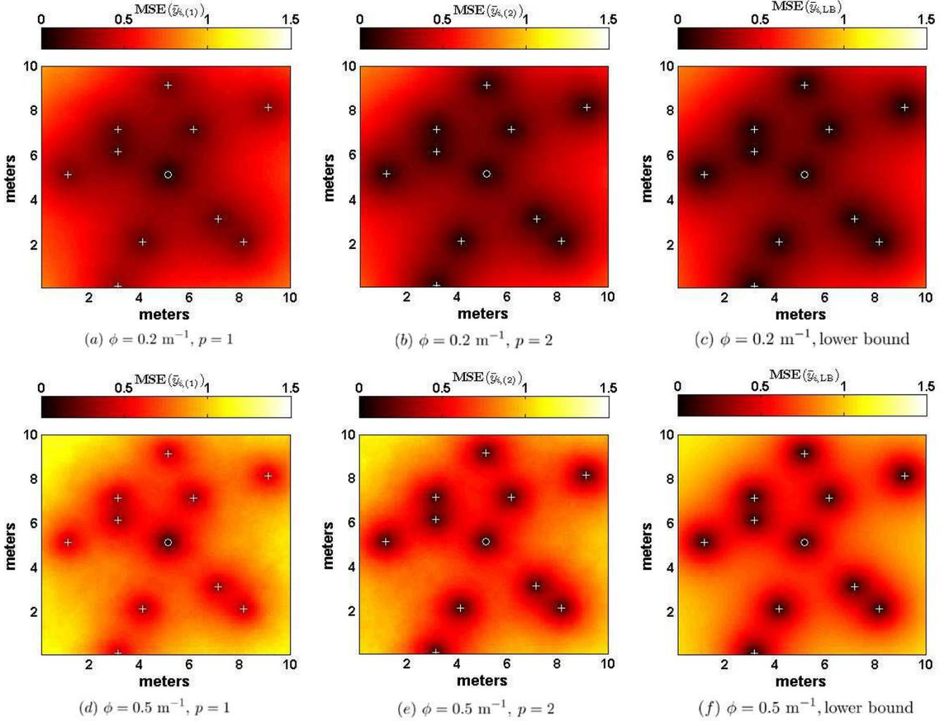
Fig. 6. Constant mean-signal scenario: average MSEs of the feedback MC random-field predictors for (a)  $\phi = 0.2 \text{ m}^{-1}$  and  $p = 1$  round, (b)  $\phi = 0.2 \text{ m}^{-1}$  and  $p = 2$  rounds, (c) lower bound for  $\phi = 0.2 \text{ m}^{-1}$ , (d)  $\phi = 0.5 \text{ m}^{-1}$  and  $p = 1$ , (e)  $\phi = 0.5 \text{ m}^{-1}$  and  $p = 2$ , and (f) lower bound for  $\phi = 0.5 \text{ m}^{-1}$ , using  $K = 3$  quantization intervals.
