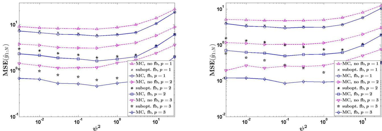
Fig. 13. Linear trend-surface scenario: Average MSEs of the proposed estimators of  $\mathbf{y}_{1:N}$  as functions of  $\psi^2$  for (a)  $K = 2$  and (b)  $K = 3$  quantization intervals and  $p \in \{1, 2, 3\}$  rounds.
