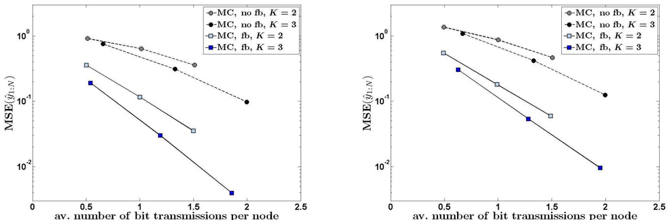
Fig. 5. Constant mean-signal scenario: Average MSEs of MC random-field estimators as functions of the average number of bit transmissions per node, for (a)  $\phi = 0.2 \text{ m}^{-1}$  and (b)  $\phi = 0.5 \text{ m}^{-1}$ .
