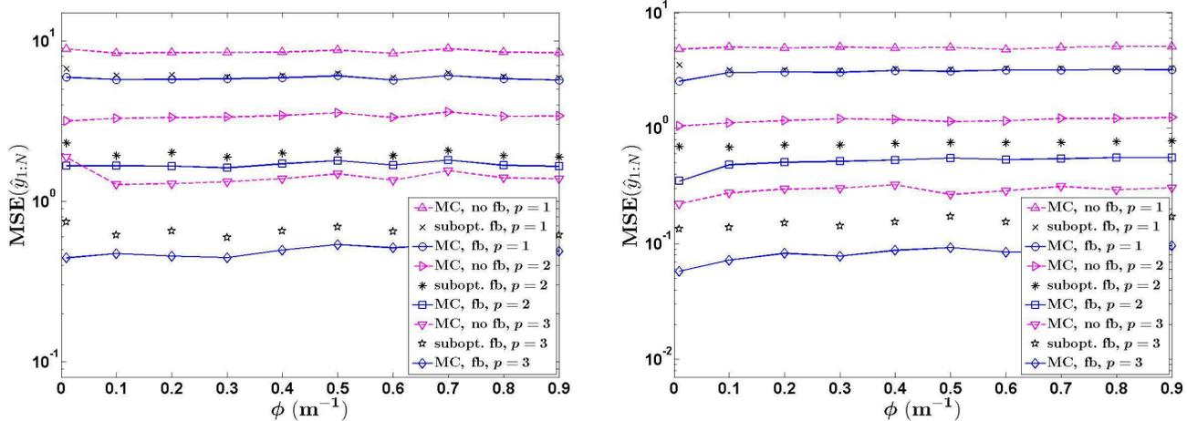
Fig. 9. Linear trend-surface scenario: Average MSEs of the proposed estimators of  $y_{1:N}$  as functions of  $\phi$ , for (a)  $K = 2$  and (b)  $K = 3$  quantization intervals and  $p \in \{1, 2, 3\}$  rounds.
