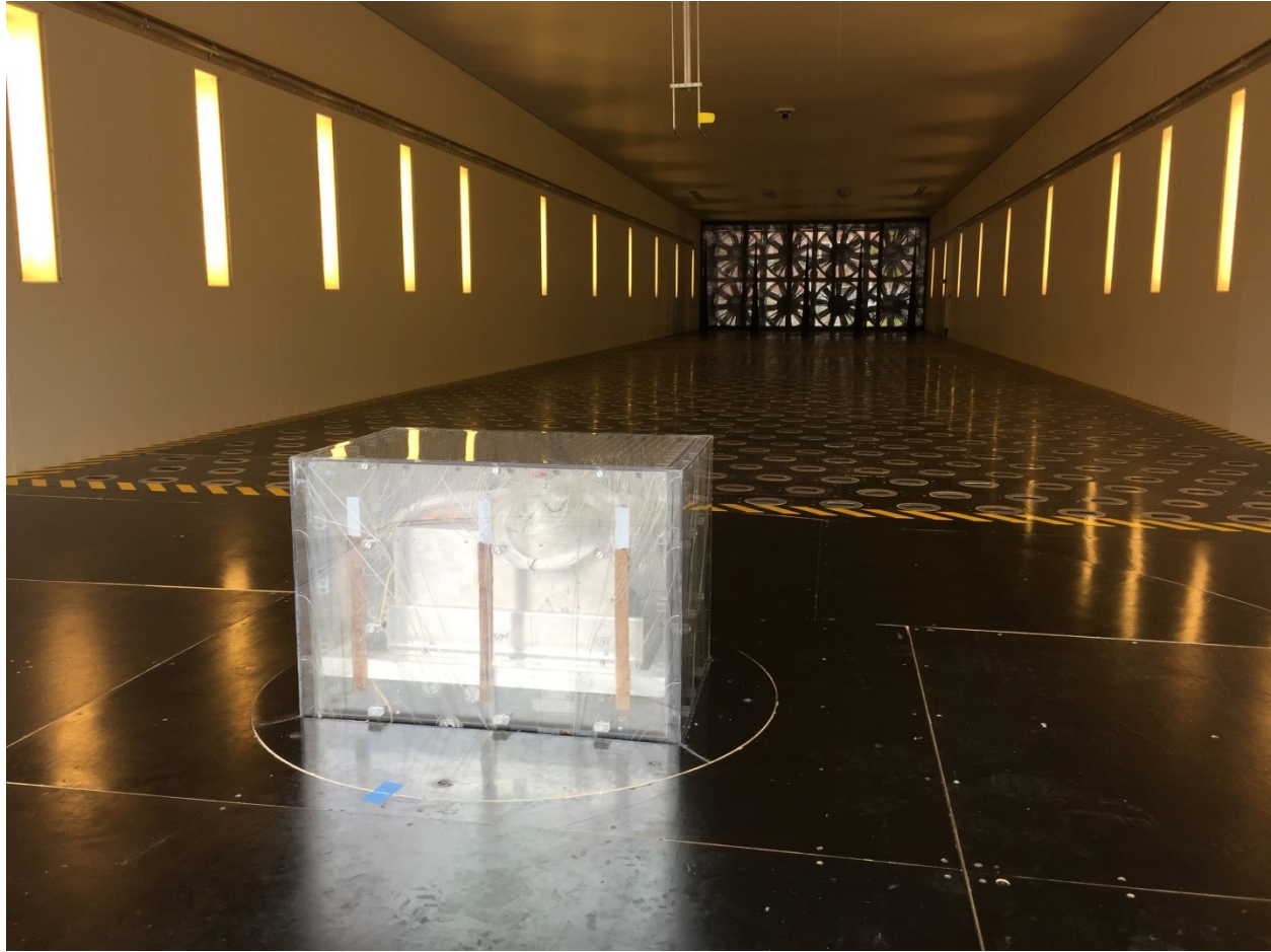
Figure 6. Boundary layer wind tunnel with model low-rise building, upwind view
