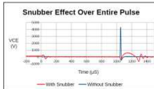
Figure 3 Comparison of IGBT collector and emitter voltage curves with and without snubber in the circuit
