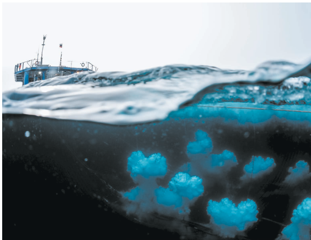
Research vessels use air guns to generate sound waves that probe the sea floor for natural resources.
