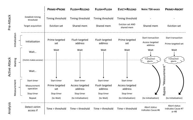
Figure 1: Comparison of the operation of various cache attacks, including our novel attacks.
