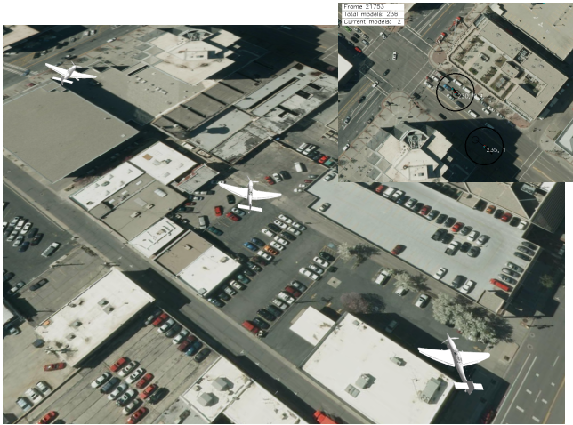
Fig. 6. A Gazebo screenshot showing multiple simulated aircraft. Simulated camera gimbal view is shown top right.
