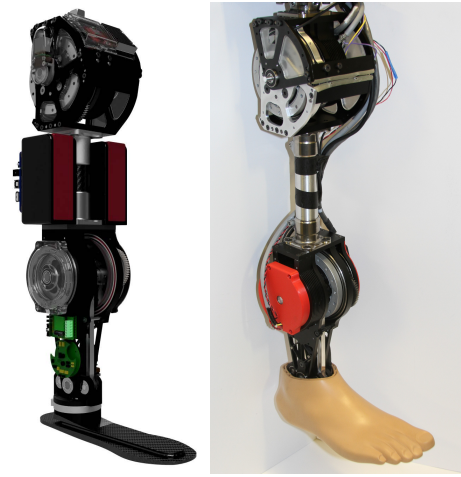
Fig. 2. Final assembly of the prosthetic leg. The image on the left displays a CAD rendering, and the image on the right displays the physical system after assembly. Note that for simplicity, certain components of the electronics system shown in the rendering are located on the benchtop for the experiments presented in Section III.
