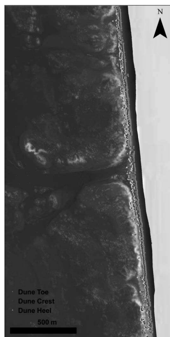
Figure 7. Relative relief defines dune features on the basis of their relative topographic position. Dune toe, crest, and heel are all defined and can be quantifiably extracted, although the cross-shore position of a feature may vary in the alongshore direction.
