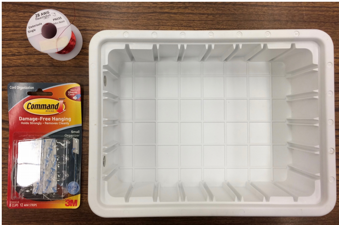
Figure 5. Components for the EclipseMob antenna.
