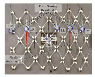
**Fig. 2.** Sensor configuration of a single segment placed flat on a surface. The FSR sensors are marked by circles around them. Stretch sensors are highlighted in red. UR: Upper Right, LR: Lower Right, UL: Upper Left, LL: Lower Left, T: Top, B: Bottom. Left and right vertex pieces join to form the ring-like structure and anterior and posterior segments are connected to the vertex pieces at the top and bottom of the figure.
