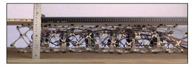
**Fig. 4.** DiSCO-Worm locomoting through two parallel horizontal wooden surfaces. The distance between the two surfaces was set at 16 cm. Both the open-loop controller and closed-loop controller were tested in the same constrained environment.
