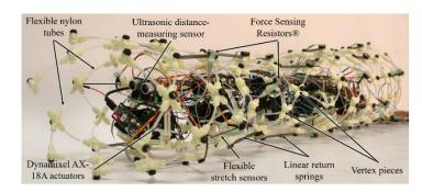
Fig. 1. Distributed-Sensing Compliant Worm robot (DiSCo-Worm) during a peristaltic wave on flat surface. The various components of the robot mesh including the sensors and actuators are labelled.
