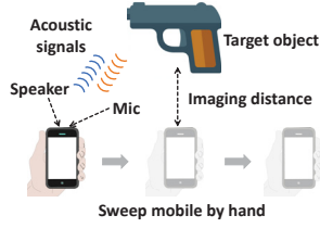
Figure 2: Smartphone based acoustic imaging.
