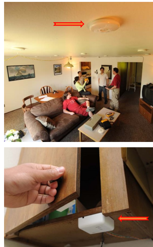
Fig. 7. Common ambient sensors monitor (top) infrared-based motion, ambient light, ambient temperature and (bottom) door open/close status. Arrows indicate a sensor location.
