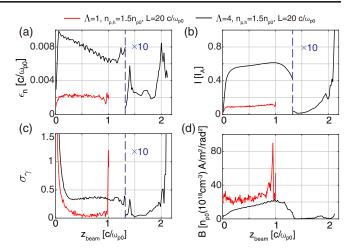
FIG. 4. The parameters of the injected beams in two conditions: (a) the slice emittance, (b) the current, (c) the slice energy spread and (d) the brightness. Here  $I_A \approx 17$  kA is the Alfven current. The beam is divided into 128 slices. The red (black) lines corresponds to  $\Lambda = 1(4)$ . The curves right of the blue dashed lines are attenuated by 10.
