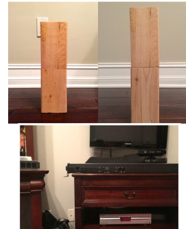
Figure 3. Image of the Wooden Block Used at 0.5-m from sensor away (top-left), 0.15-m away from sensor (top-right) and the room wall, 1.83-m away from sensor (bottom).
