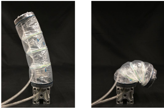
Fig. 14: Demonstration of a length-controlled bending device where the outer chamber is separated into three chambers that run the length of the device. One of these three outer chambers is pressurized. On the left, the pressure in the inner chamber is positive, while on the right the pressure in the inner chamber is negative. When the device is long, the pressurized outer chamber exerts a contractile force; when the device is short, the inflated outer chamber exerts a pushing force, reversing the curvature.
