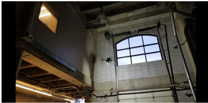
Fig. 8. An obstacle detection test for the Guidance system is shown in a maintenance bay at Montana Tech. In this instance, the Guidance is preventing the M100 from colliding with the wall.
