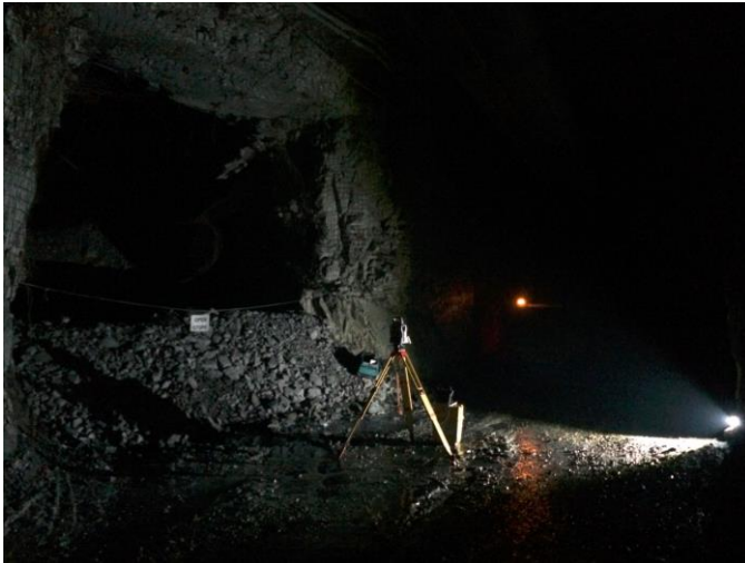
Fig. 11. Total station set up at the entrance to the 'NEV' stope on the 4305 level. The total station had to be within line-of-sight of the survey control points and paintball marks within the stope.
