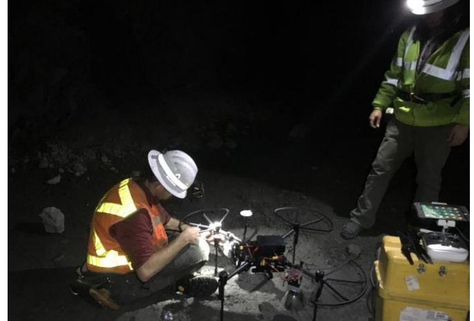
Fig. 2. The M100 underground at the Barrick Golden Sunlight Mine with a standard payload of lights, a camera, and the Guidance system.
