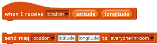
Fig. 4. Sending and receiving messages with data in NetsBlox.
