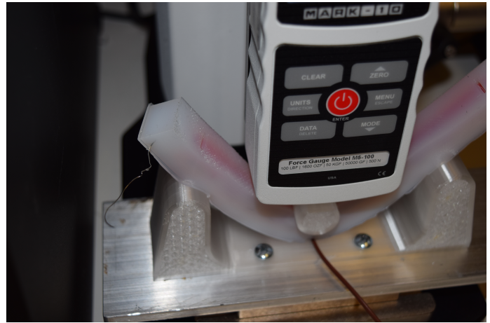
FIGURE 8. Twisting behavior of Nitinol/PCL composite beam under loading of bend test above melting temperature of PCL.
