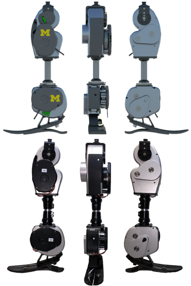
Fig. 1. Rendering (top) and physical implementation (bottom) of the OSL.
