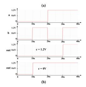
Figure 1: Polymorphic AND/OR gate. (a) Topology (b) Input and output waveforms (from top to bottom: input a, input b, output with c = 1.2V, output with c = 0V).
