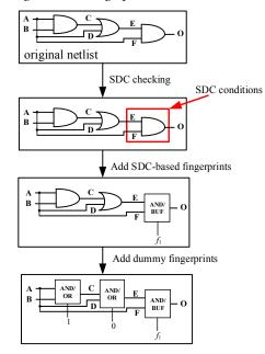
Figure 3: Design flow of the proposed scheme
