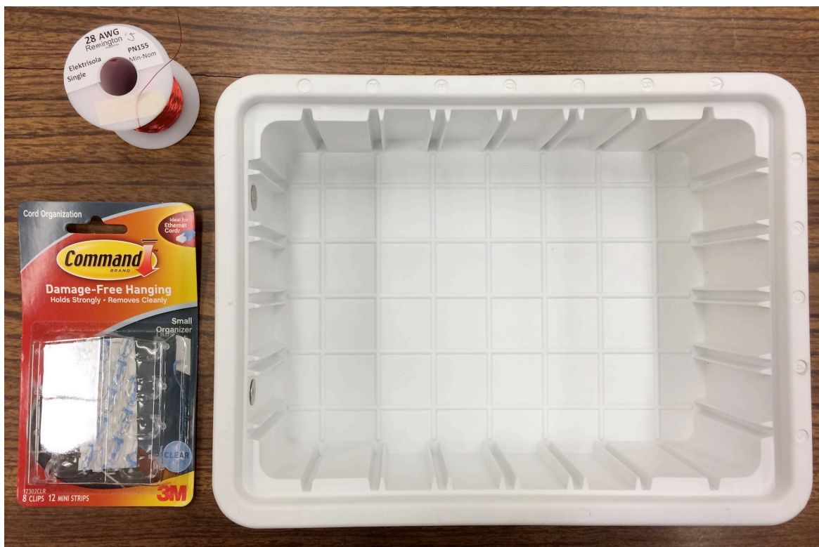
Figure 5. Components for the EclipseMob antenna.
