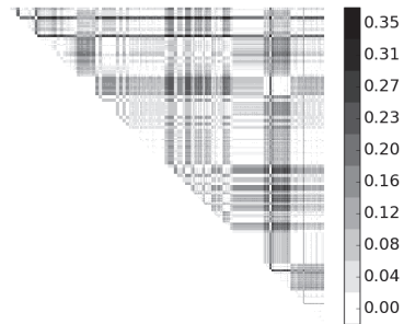
(b) Similarity matrix of interval error rates for ten benchmarks. The diagonal of matrix represents the execution of benchmarks concatenated. Each point is the error rate difference between two intervals (projected horizontally and vertically to the diagonal). The darker, the more different.
