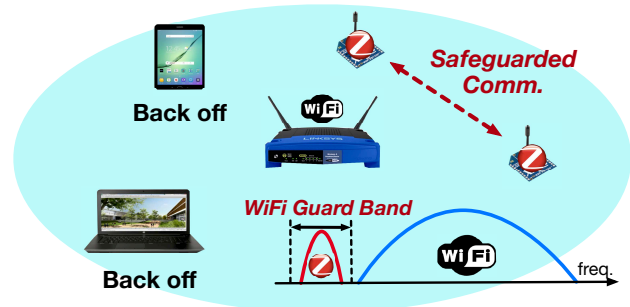
Figure 1: Our system places ZigBee transmission (red) in the guard band of ongoing ambient WiFi (blue). This essentially safeguards ZigBee from the WiFi interference, as WiFi devices in proximity back off as per CSMA.
