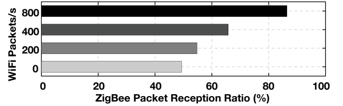
Figure 3: WiFi traffic (@ Ch_1^w ) vs ZigBee PRR (@ Ch_{15}^z ).
