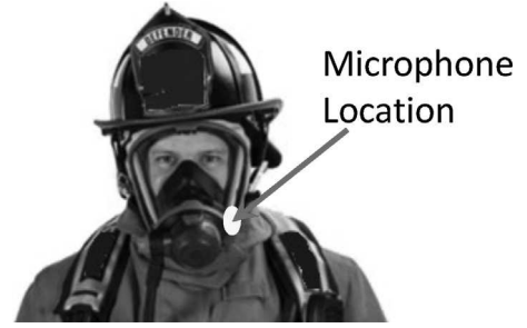
Fig. 6. Placement of impromptu data collection system on outside of the firefighters SCBA mask [18].
