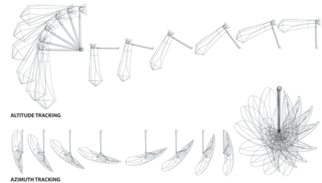
Figure 4. Heliotropic two-axis tracking of louver modules.
