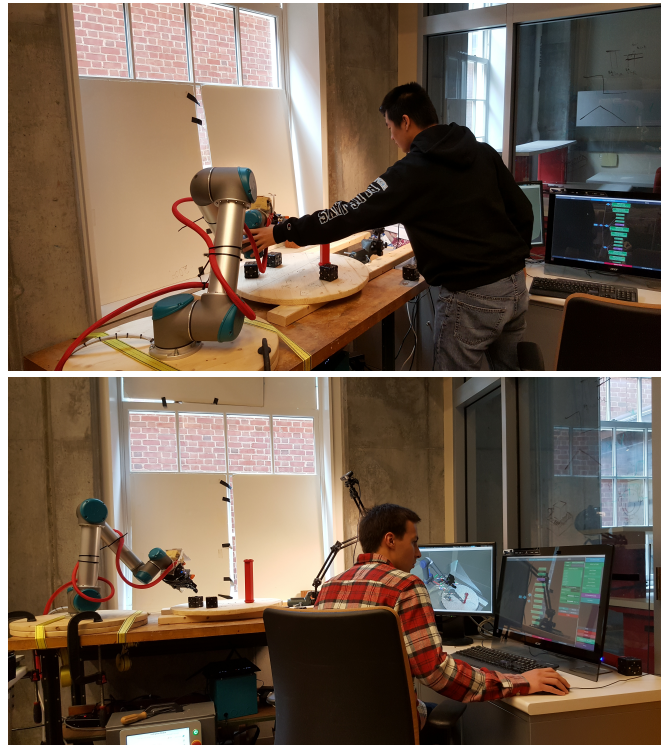
Fig. 1: Users interacted with the CoSTAR system in different ways. Left: a user positions the robot to teach it a new waypoint. Right: a user fine tunes part of a tree using the BT-based user interface.
