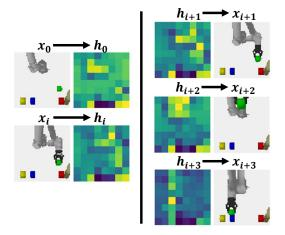
Figure 1: Example of our algorithm using learned policies to predict a good sequence of actions. Left: initial observation  $x_0$  and current observation  $x_i$ , plus corresponding encodings  $h_0$  and  $h_i$ . Right: predicted results of three sequential high level actions.
