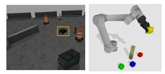
Figure 6: Simulation experiments. Left: Husky navigation task. The robot is highlighted. Right: UR5 block-stacking task with obstacle avoidance.
