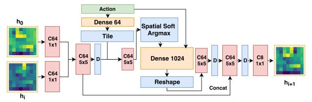
Figure 5: Architecture of the transform function  $T(h_0, h, a)$  for computing transformations to an action subgoal in the learned hidden space.
