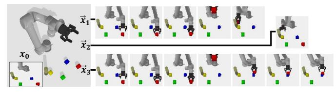
Figure 9: First three results from a call of the planning algorithm on a random environment using Alg. 1. The first two are correctly recognized as failures before the system finds a sequence of actions with high predicted values.
