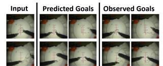
Figure 2: Predicting the next step during a suturing task based on labeled surgical data. Predictions clearly show the next position of the arms.
