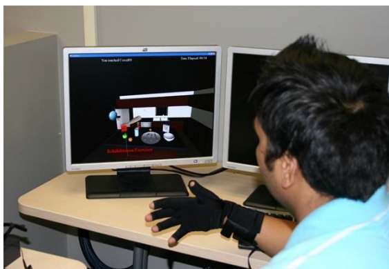
Figure 21: Real-time hand deformation using 5DT data glove
