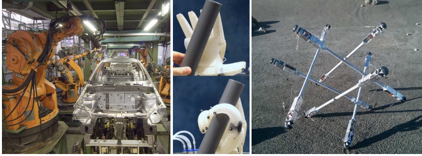
Fig. 1 Left: Rigid industrial robots for manufacturing [KUKA]. Center: a soft robotic hand conforming to a grasped object [7]. Right: NASA’s terrain-compliant tensegrity rover, SUPERball [22].
