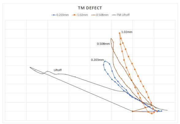
Figure 6: Results of the surface-breaking defects (cracks) in TM SS 17 4 PH sample using 500 kHz absolute frequency probe.
