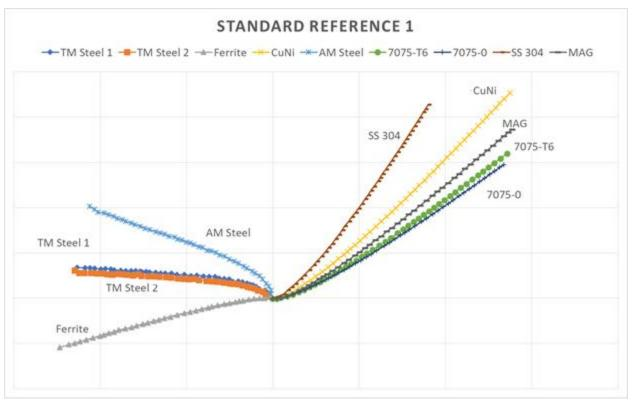
Figure 4: Lift-off curves for comparison of the conductivity for standard conductivity sample set as well as TM and AM SS 17 4 PH samples.
