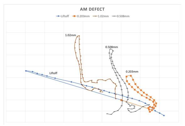
Figure 7: Results of the surface-breaking defects (cracks) in AM SS 17 4 PH sample using 500 kHz absolute frequency probe.
