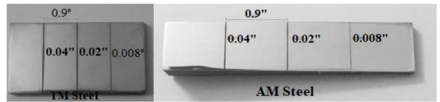
Figure 2: The TM (left) and AM (right) samples after grinding and polishing.
