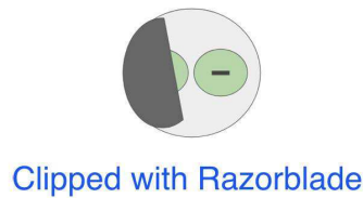
Figure 11: The phase of a clipped beam, which disrupts the symmetry at the photodiode so it will witness more higher order modes.
