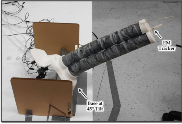
Figure 7. 45-degree tilt test set-up. EM tracker is inserted in the end cap, optical sensors and pneumatic tubing are connected at base. The EM transmitter is located approximately 10 cm away on a nonmetallic table.
