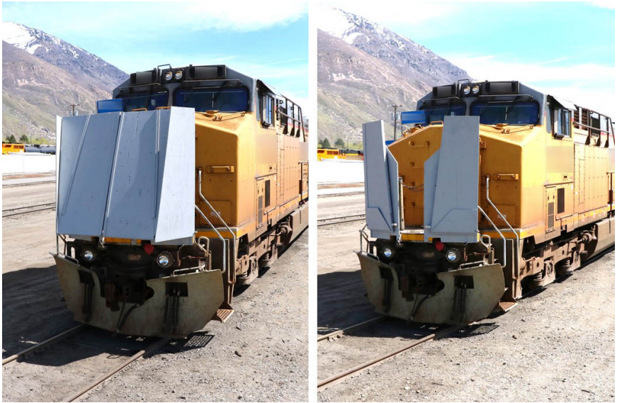
Figure 15: Full-scale prototype on a freight locomotive shown in both the stowed configuration (right) and deployed configuration (left). Photo has been modified to remove locomotive identity.
