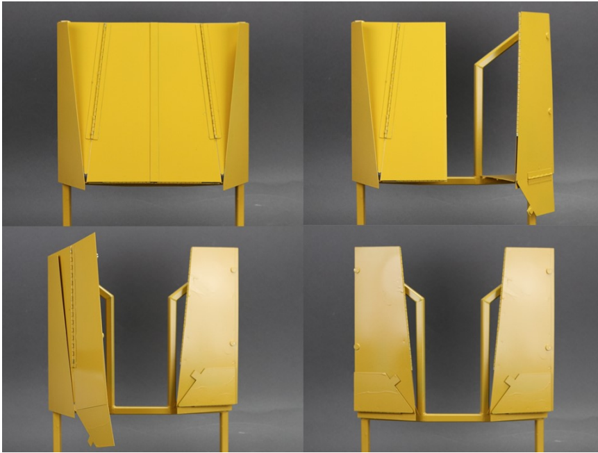
Figure 14: Eighth-scale prototype constructed from sheet metal.
