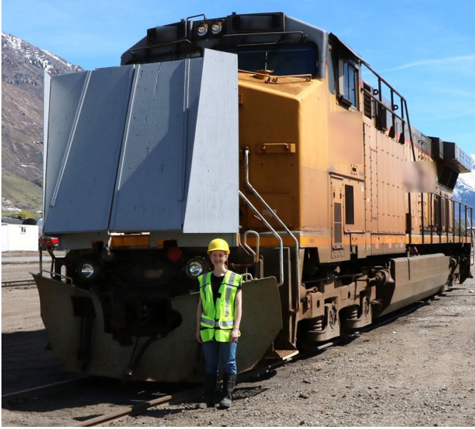
Figure 16: The top of the fairing is 3.6 meters above the ground. An 159 cm tall person provides a visual indication of the fairing size. Photo has been modified to remove locomotive identity.
