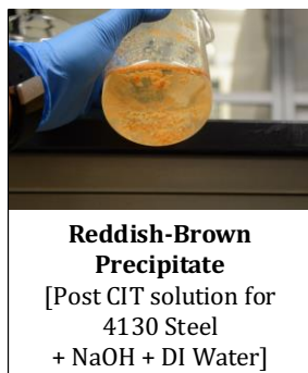
Figure 6: Chemical analysis to show etching effect that brought Fe elements to the solution.
