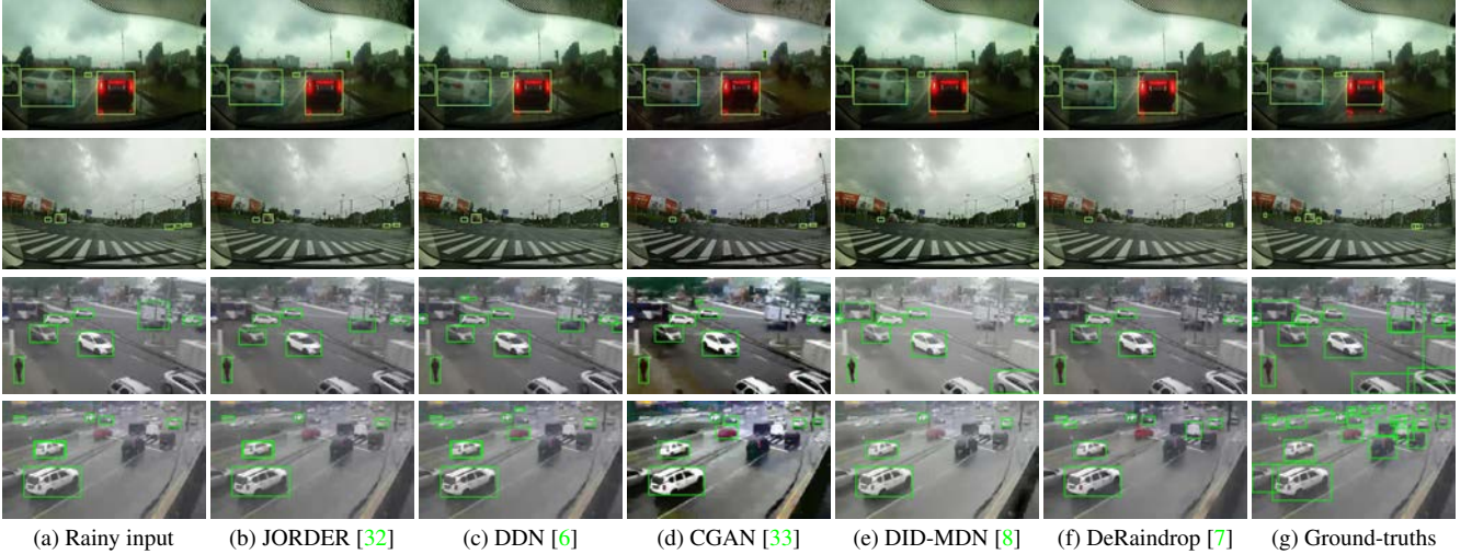
Figure 3. Visualization of object detection results after applying different deraining algorithms on two images (first two rows) from the RID dataset and two examples (last two rows) from the RIS dataset.
