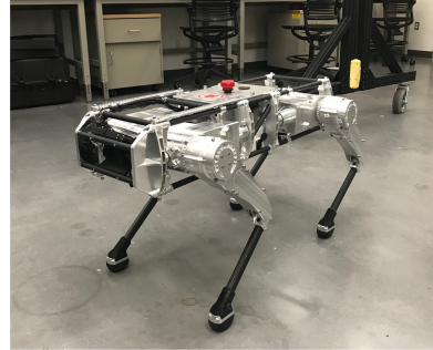
Fig. 1: Vision 60, a 3D quadruped robot with 18 DOFs, designed and manufactured by Ghost Robotics [46].
