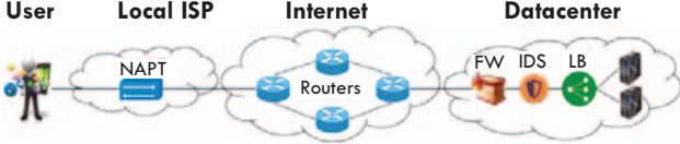
Figure 2. A typical service function chain in telecommunication data centers. The user traffic will be processed by firewall, DPI and load balancer sequentially.
