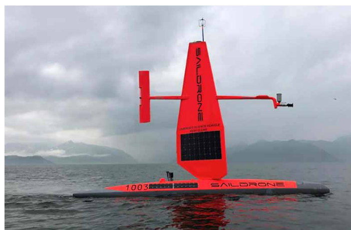
Figure 1. A Saildrone deployed off the coast of Alaska, with a three-axis sonic anemometer at the top of the sail, along with temperature, humidity, and radiation on a forward probe. Image credit: Saildrone Inc.
