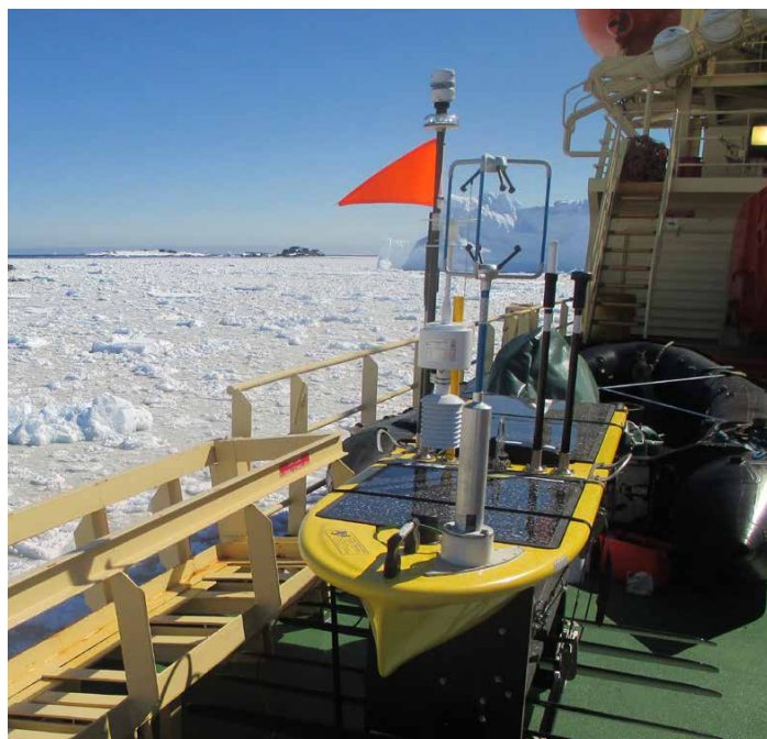
Figure 2. A Wave Glider before deployment off the Antarctic Peninsula, with a three-axis sonic anemometer at the bow, along with temperature, humidity, and pressure sensors on a mast. Image credit: Avery Snyder (APL-UW)
