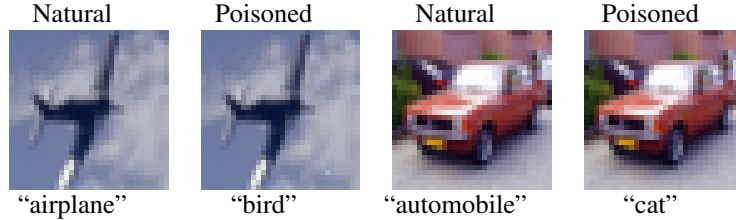
Figure 2: Examples of test images on which the model evaluates incorrectly with the presence of a backdoor. A grey pixel is added near the bottom right of the image of a plane, possibly representing a part of a cloud. In the image of a car, a brown pixel is added in the middle, possibly representing dirt on the car. Note that in both cases, the backdoor (pixel) is not easy to detect with the human eye. The images were generated from the CIFAR10 dataset.
