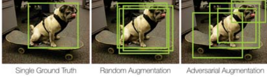
Figure 2. Types of annotation distributions. Adversarial augmentation selects bounding boxes that are maximally different from the ground truth but still contain important object features.
