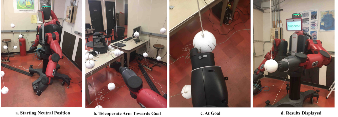
Figure 2: The steps of a task in our testing sequence from a pointing dataset [30] include starting from the robot’s neutral position (a) and then teleoperating the arm of the robot (b) to the goal location (c) at which point confirmation is displayed on the robot’s screen (d).
