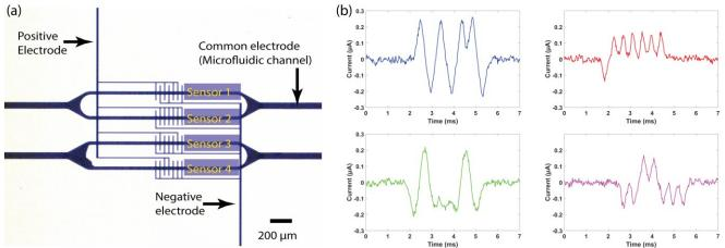
Figure 5: Microfluidic CODES device formed by parallel electrodes and the resulting representative signals from individual sensors. (a) A close-up image of the 4-sensor Microfluidic CODES device fabricated by the reported method. Sensors are encoded with orthogonal digital codes "1010110", "0111111", "0100010", "0011000", respectively. (b) Representative signals corresponding to each sensor in the device shown in (a).
