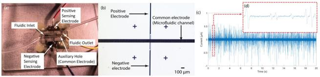
Figure 3: Images of the fabricated microfluidic device and characterization results. (a) A photo of the fabricated device with fluidic and electrical connections and (b) a close-up of the parallel electrode sensor. (c) Approximately 2500 cancer cells were detected by the sensor during 20 s period. (d) A close-up figure showing the signals for 7 detected cells in 0.04 s.
