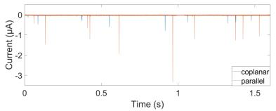
Figure 4: Resistive pulses recorded from a coplanar-electrode and a parallel-electrode sensor sequentially placed on the same microfluidic path with a 15  $\mu$ m channel height. The peak signal amplitudes generated due to the same cell are on average ~3.7× higher for the parallel-electrode sensor. The result was found to be consistent with the finite element analysis results (not shown).
