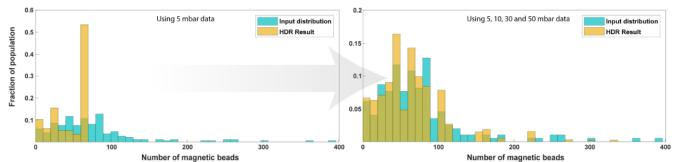
Figure 3: Improvement of the HDR results with additional information from different flow rates. The effective dynamic range of the system increased by collectively analyzing the aggregate data from different flow rates.
