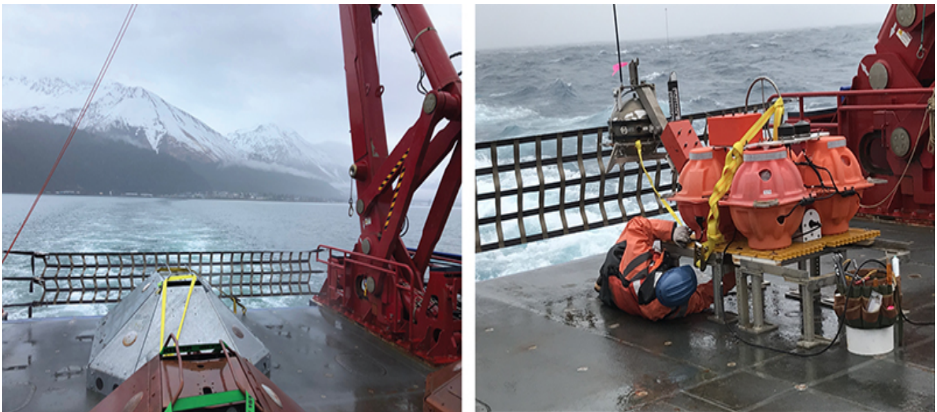
Fig. 2. Ocean bottom seismometers used in AACSE. A shallow-water instrument (left). Dan Kot
