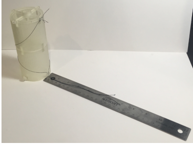
Fig. 12. Geometric model validation test set-up. The length change of the cables was measured with a ruler. Twist was measured via indentations in the rotary joint placed every 5° on both the base and top.
