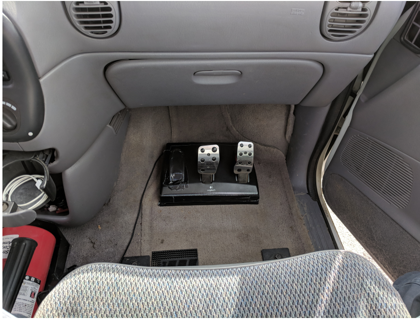
Figure 4 G27 Gaming Pedals that were used to mediate participants' inputs.
