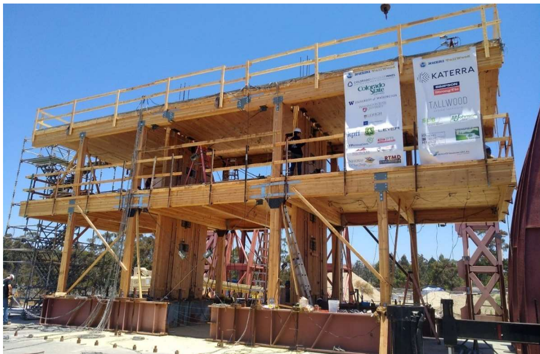
Figure 4. Fully constructed test building on steel foundation connected to the shake table.
