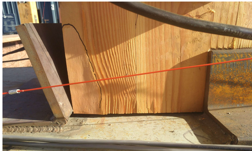
Figure 6. Observed damage to rocking wall corner after MCE level test.
