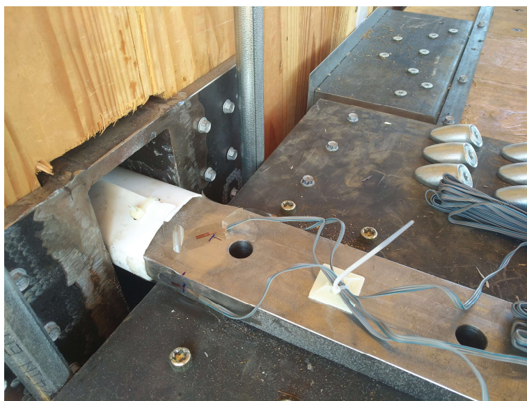
Figure 7. No damage at the wall-diaphragm shear transfer connections.
