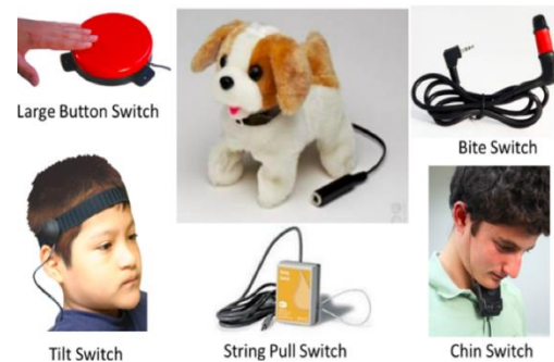
Figure 1: Adapted toy and sample activation switches: The dog is an example of an adapted toy with a universal activation port. This adapted toy can be activated by a variety of alternative activation movements including pushing a large button, tilting one's head, pulling a string, biting, or pushing one's jaw downward. This figure is from our previous work [3] and some images are from [4-5].
