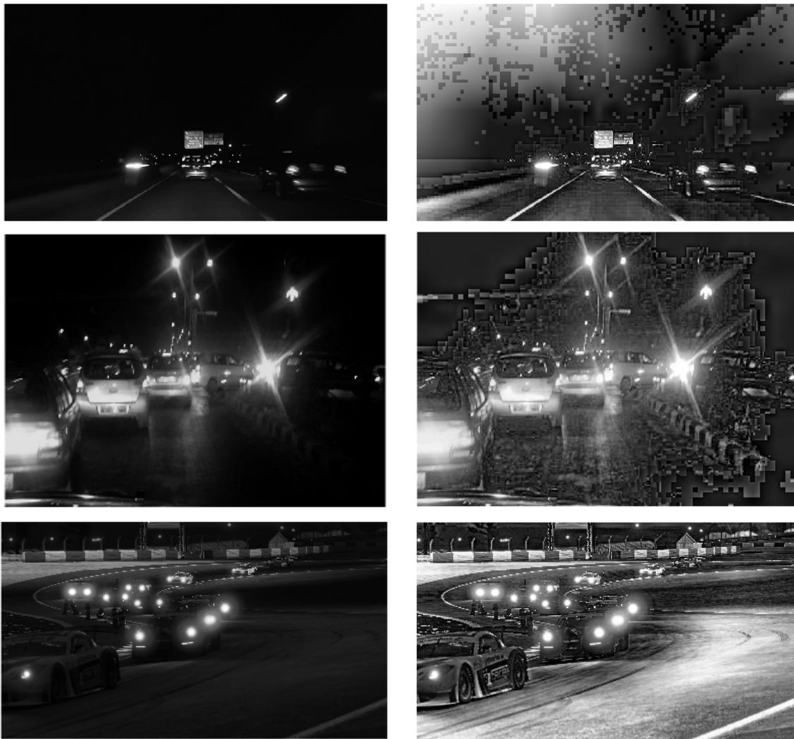
Figure 5: Examples of three images used in an object detection experiment using the proposed method. All three original inputs are shown on the left column and have been retrieved from a public internet image database. In all of them visibility is reduced due to low and uneven illumination. Top and middle originals have been encoded with a lossy compression JPEG. Lossless compression has been applied to the bottom original. In the right column you can observe the outputs of \mathcal{IN} for each one of the originals. The pixelization appearing mostly where the original images are dark is the result of the enhancement of pixelization existing in the input images. We show this in Fig. 6. Observe that the output of the bottom image does not have these artifacts.
