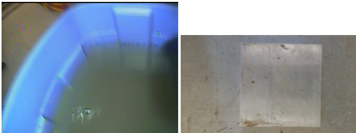
Figure 12: High turbidity simulation experiment in a small tank. The water depth is 9.5in. The metal plate shown on the right panel was resting on the bottom of the tank.
